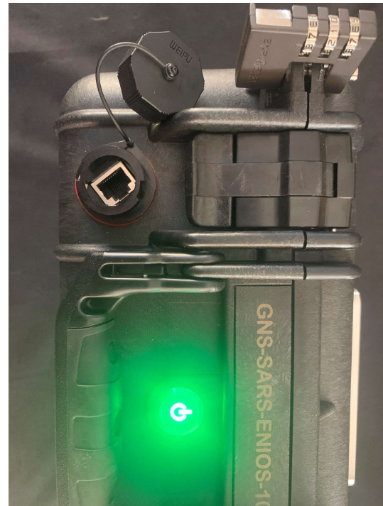
Figure 5: Connecting UTP Cable To Mobile Case
